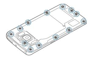
4 Remove the circuit board.
