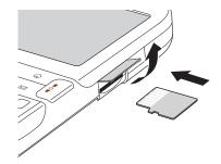
4 Insert the microSD card into the microSD expansion card slot until you feel it lock into place.
