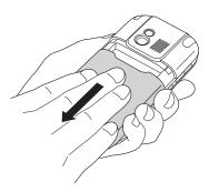
2 Align the metal contacts of the battery with the smartphone contacts inside the battery compartment, and press the battery into place.
