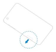
Hold the nano-SIM card/ microSD card with the cut corner oriented as shown and slide it into the card slot
