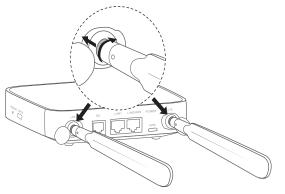
③ Screw external antennae fully into the antennae ports.
