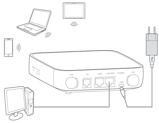
To prevent interference caused by radio signals, place the Cat4 Router at least one meter away from phones and other electrical devices.
