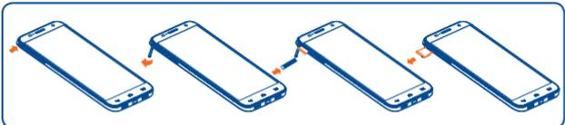
Insert the microSD card with the golden contact facing downwards into the slot. To remove the microSD card, gently press and slide it out.
