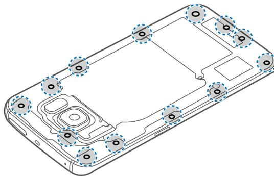
4 Remove the circuit board.
