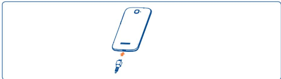
Connect the battery charger to your tablet and mains socket respectively.
