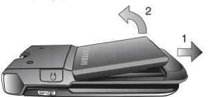
2. Grip the battery at the bottom and pull up and out at a 45° angle.
