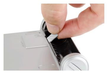
**9** Push the top of the SIM card firmly until it clicks into place in the card slot.
