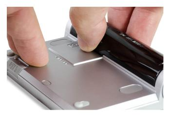
**3** Using normal thumb pressure on the thumb notch, lift the battery door up to remove the door completely.
