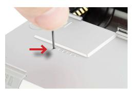
Insert a paper clip into the hole and hold the button down for five (5) seconds.
