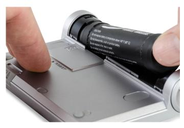
**2** Push firmly to snap the battery into place.
