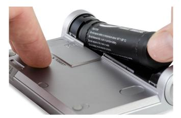
**6** Lift the battery out of the battery well.
