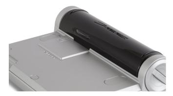
2 Steady the MiFi 2 with one hand and place the thumb of your other hand on the battery door thumb notch.
