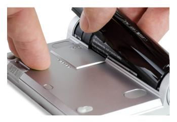
**4** Use your forefinger to pull the battery up slightly so that it moves out of the battery well.
