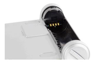
4 Hold the card with two fingers and insert into the SIM card slot, being careful not to touch the gold contacts on the back of the card.
