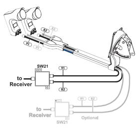
satellite signal. Whichever multi-dish switch that is left un-used will be available in case you wish to connect a second satellite receiver in future.
