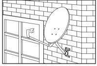
You can mount the satellite antenna on a solid brick wall.
