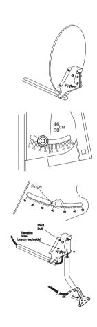
Tighten the mast clamp bolts so that the clamp is snug, but can still be moved back and forth.
