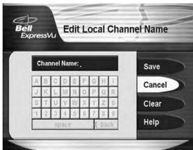
Highlight a letter and press the SELECT button. Do this again to spell out the channel name. You can enter up to five characters. If you need to, use the space option to insert a **space** or the **<back** option to correct a letter. When you are done entering the channel name, select the **Save** option. This opens the **Local Channel Setup** menu again.
