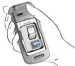
5. Replace the battery and the cover. Turn the battery cover screws clockwise to lock the battery cover.
