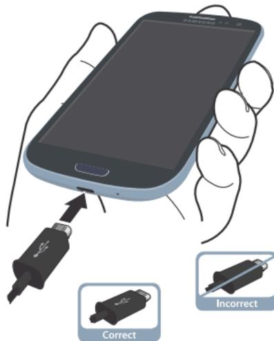
1. Plug the flat end of the Travel Charger into the Power/Accessory Interface connector and the other end into a standard AC wall outlet.
