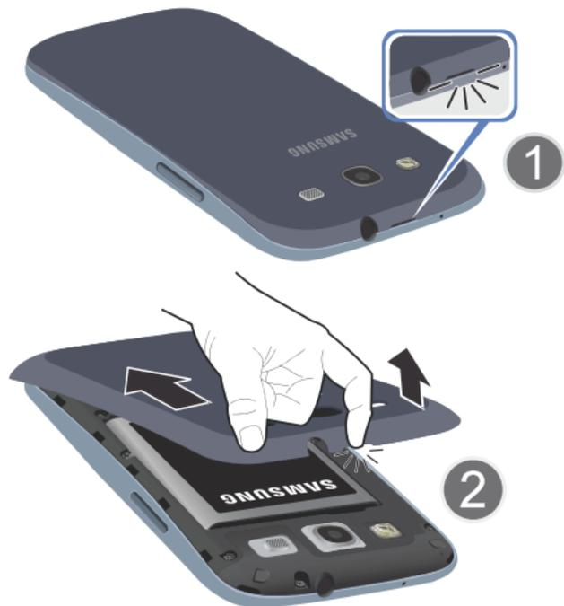
3. If necessary, remove the battery.
