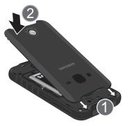
2. Press along the edge of the back cover (3) until you have a secure seal.
