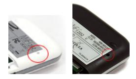
Insert a paperclip into the hole and hold the button down for 5 seconds until the LED goes off.
