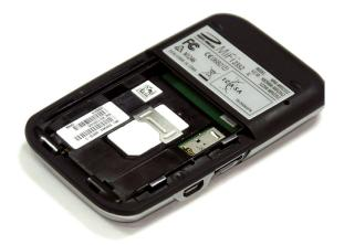
• Now, insert the battery, lining up the contact points as shown and replace the door on the device.
