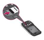
2 Insert the memory card into the slot. Make sure the gold contact area is facing downwards.
