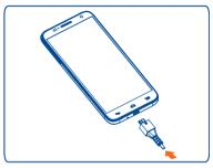
Connect the battery charger to your phone and mains socket respectively, the LED indicator will light while charging.
