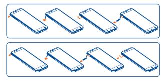
Insert the microSD card with the golden contact facing downwards into the slot. To remove the microSD card, gently press and slide it out.
