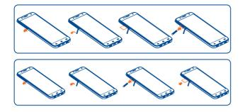
To install, place the SIM card with the chip facing downwards in to the housing, and then slide it into its slot. Make sure that it is correctly inserted. To remove the card, press and slide it out.
