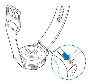
2 Slide the spring bar inwards and connect the band.
