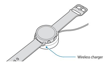
3 After fully charging, disconnect the Galaxy Watch Active2 from the wireless charger. Disconnect the wireless charger from the charger and then unplug the charger from the electric socket.
