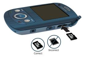
**Note**: To remove the card once it has been inserted, firmly push the end of the card further into the phone and release—the card should pop out of the memory card slot. If this does not work, repeat the process again.
