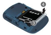
Insert the top end of the battery cover into the grooves of the phone. Snap the lid into place.
