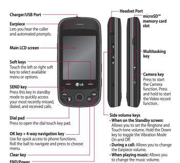
Ends or rejects a call. Turns the phone on/off. Press once to return to the standby screen.
